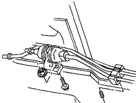
**The Fuel Filter Is Located On The Drivers Side Sub Frame Forward Of The Fuel Tank**
